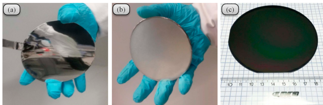
Figure 2. Photographs of a 4-in. wafer-scale Al foil after surface polishing for UTAM preparation (a), as-prepared UATM on the Al foil (b), and the UATM transferred on a Si wafer (c).
